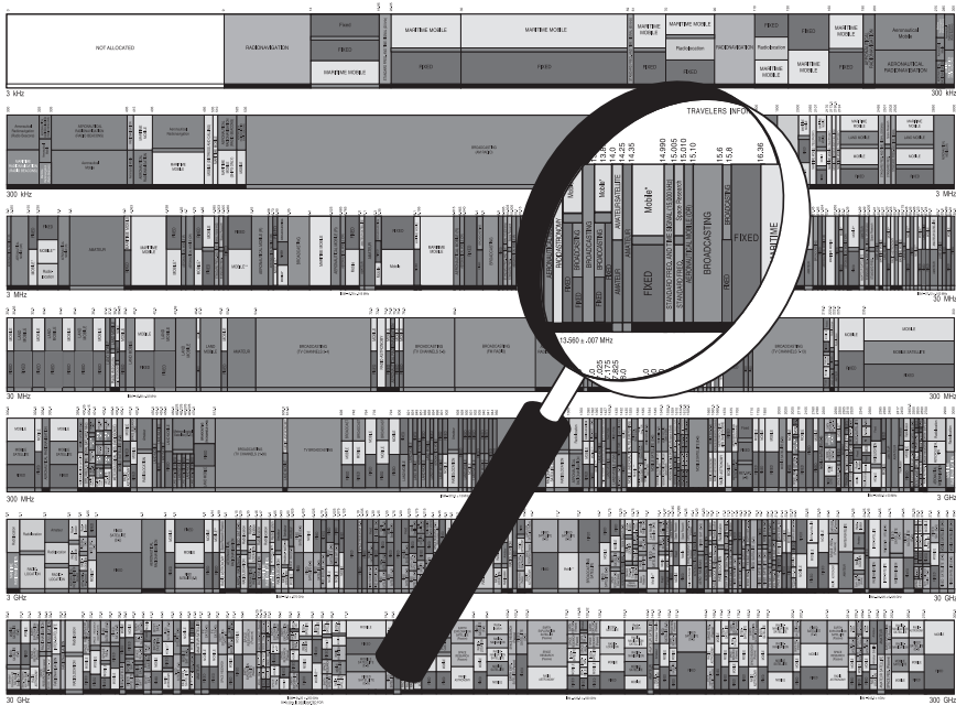
FIGURE 8.1 Frequency allocation of the U.S. radio spectrum. The spectrum from 3 kHz to 300 GHz is laid out from left to right and top to bottom, with the scale 10 times denser in each successive row. For example, the large block in the second row is the AM radio dial, about 1 MHz wide. The same amount of spectrum would be about .00002 inch wide in the bottom row. 9
