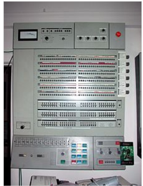
An IBM System 360/65 Operator's Panel. OS/360 was used on most IBM mainframe computers beginning in 1966, including computers used by the Apollo program .
