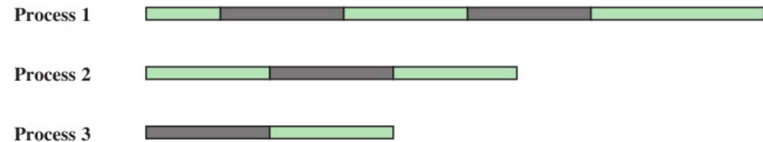
(b) Interleaving and overlapping (multiprocessing; two processors)
